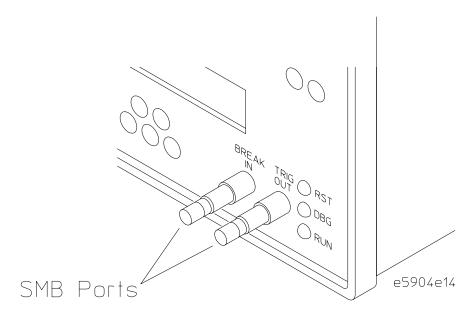
By using the FPGA trace port analyzer's "trigout" and "breakin" configuration options, you can route the Trigger Out and Break In signals to either the JTAG unit or to the trace port analysis unit.
