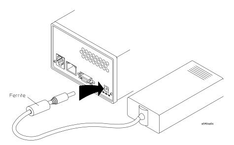
Ensure the power supply plug is completely seated in the power input receptacle.
