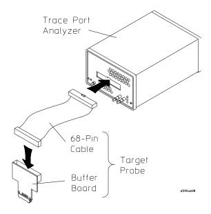
Step 4. Plug the target probe into the target system MICTOR header connector.
