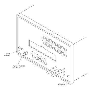
The green LED, to the left of the power switch, is lit when the FPGA trace port analyzer is connected to a power source and the power switch is on.
