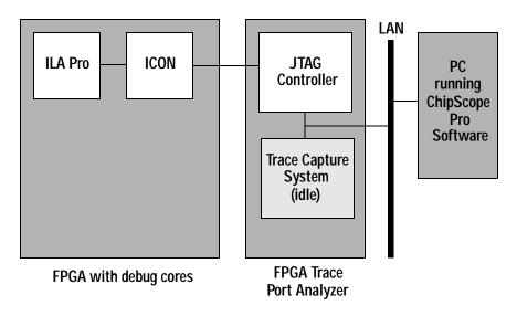
2. Xilinx ICON with ILA Pro and Agilent Trace Core (ATC) when Agilent's FPGA Trace Port Analyzer is used for trace memory.
