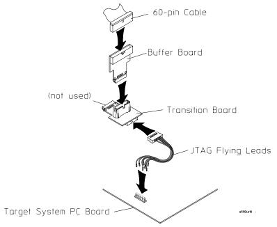
• The target system has a MICTOR for trace, but the JTAG lines were not connected to the MICTOR.
