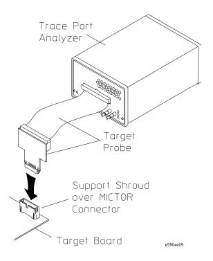
Step 5. Turn ON the FPGA trace port analyzer power switch.
