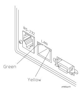
The yellow LED, on the right side of the connector, indicates LAN activity (receive or transmit).
