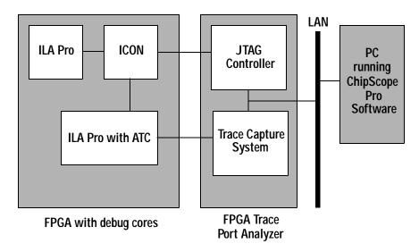
Xilinx ChipScope Pro provides the user interface to the ILA Pro with ATC. It configures the on-chip debug cores using a JTAG controller. ChipScope Pro also displays trace captured by the FPGA Trace Port Analyzer.
